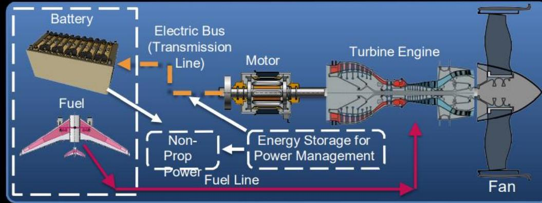
Both concepts can use either non-cryogenic motors or cryogenic superconducting motors.
