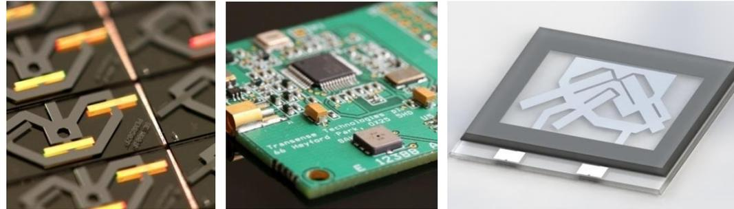
Measures strain, pressure, torque, thrust and temperature using Surface Acoustic Wave (SAW) resonators.
