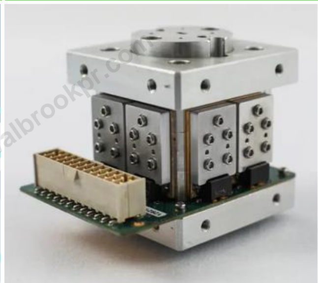
Exhibit 7: Cerus power amplifier for high-capacity point-to-point satellite and HAPS applications
