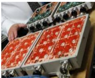
Switch Filter banks
