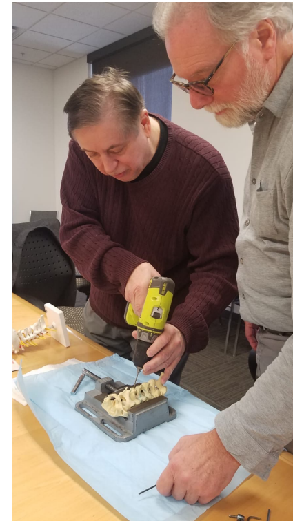
Professor Boehm with saw bone saw bone testing with traditional pedicle screw
